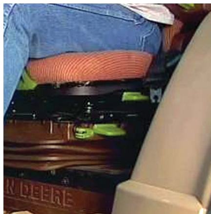
Figure 5. Retrofitted tractor seat for protecting operators with certain disabilities.
