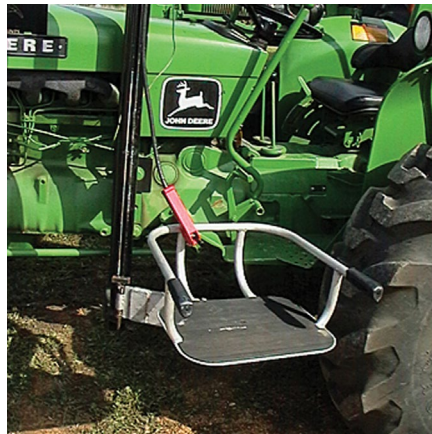
Figure 2. Left, tractor retrofitted with additional steps; right, tractor equipped with mechanical lift.
