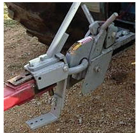
Figure 6. Quick connect adaptor for attaching and detaching implements to the drawbar.
