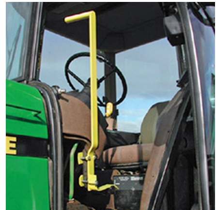
Figure 3. Hand-control linkage for operating the clutch.
