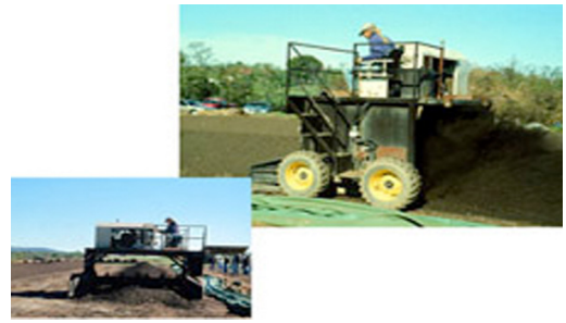
Windrow turner--mixes and aerates compost.
