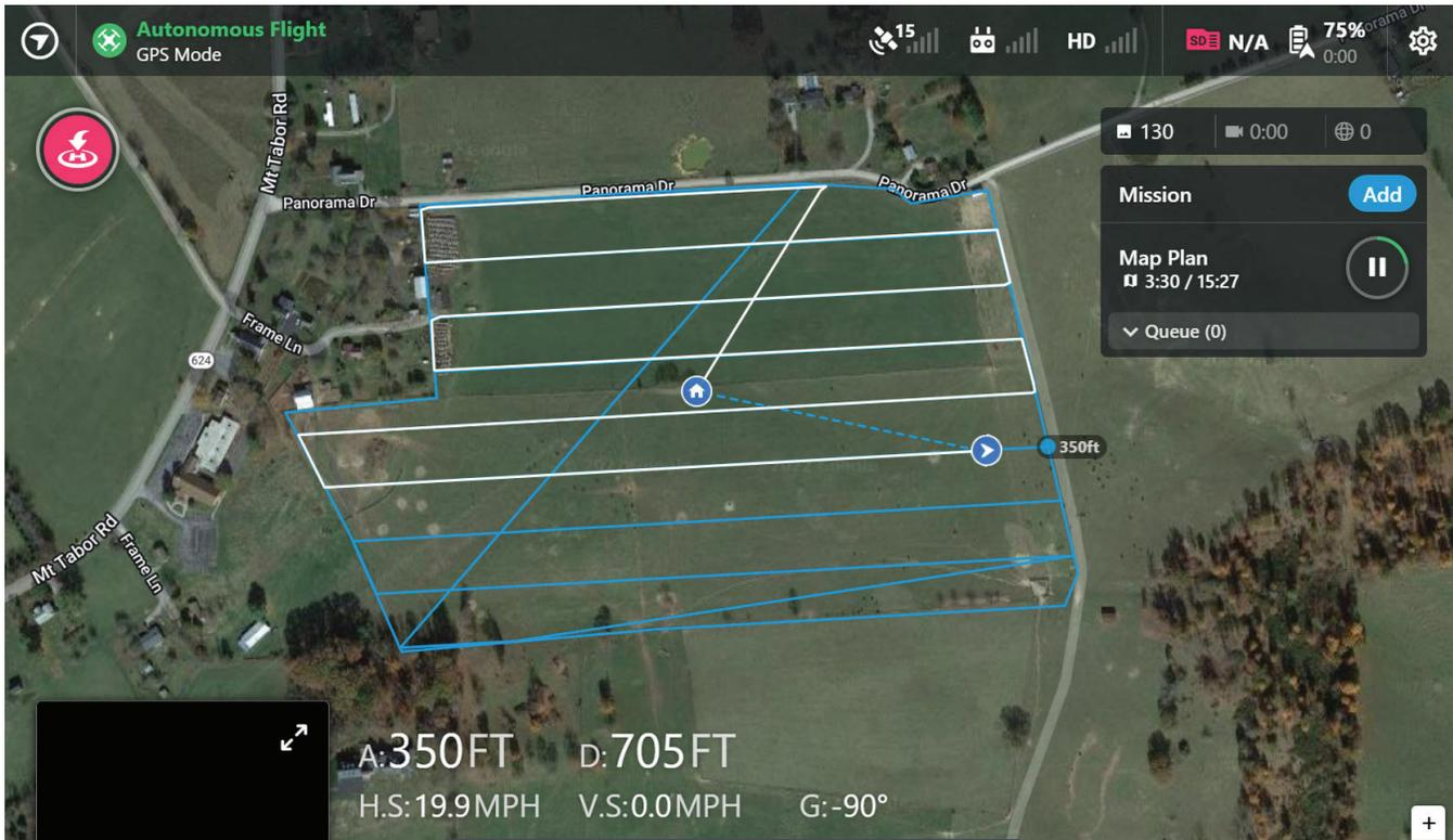
Figure 39: DroneDeploy screenshot taken during a mission.
