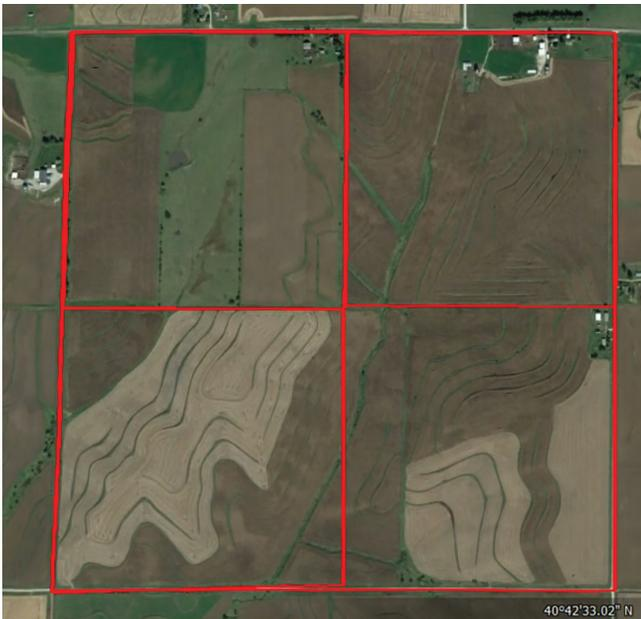
**Figure 2:** An outline of a PLSS section and quarter sections.
