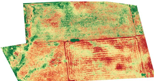
**Figure 55:** VARI image produced by DroneDeploy of the hay and pasture fields from figure 53.
