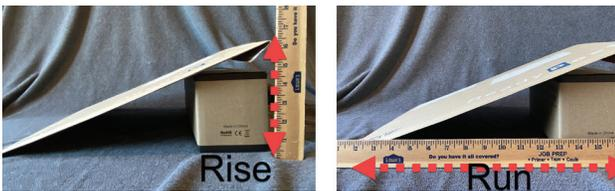
**Figure 3:** Measuring the rise and run of a slope.
