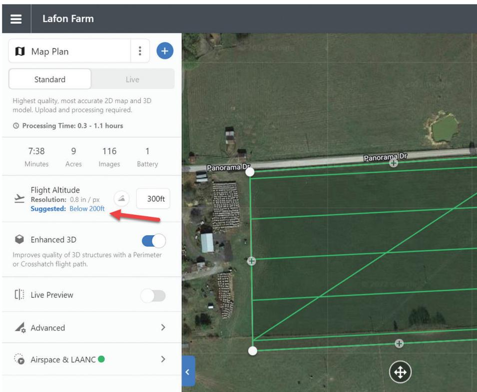
**Figure 34:** Autonomous Flight Planning in DroneDeploy.
