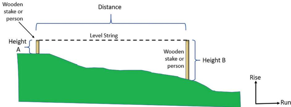
**Figure 4:** Determining slope in the field. Note that a small string level can be used to ensure that the string is level (or you can eyeball it).
